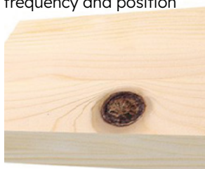
Knots: their type, size, frequency and position
